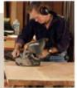
Watch chip output to determine flatness. Set the planer to a lighter cut. If the surface is flat, the planer should send out a steady stream of fine shavings.
