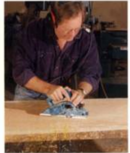
Watch chip output to determine flatness. Set the planer to a lighter cut. If the surface is flat, the planer should send out a steady stream of fine shavings.
