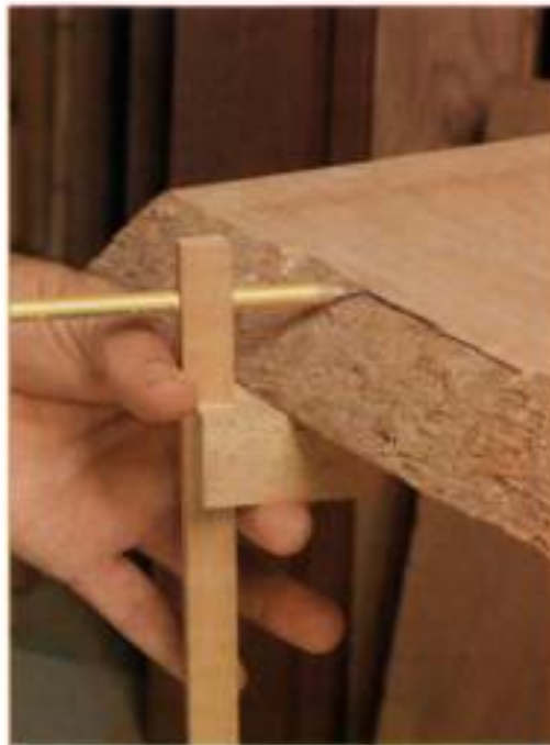
Scribe 1/16 in. over final thickness. Pick a show face and scribe from the bottom of the plank for your final passes with the power planer. Hare uses a shopmade marking gauge to work around live edges.
