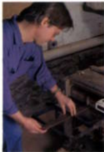
Mark stock before cutting plies. Plies are numbered (above) so they won't get mixed-up as they are band-sawn and then run through a thickness planer (right).
